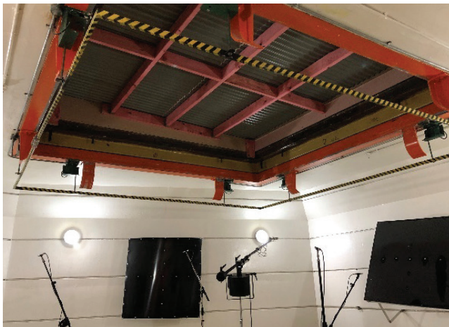
Test setup mounted within a diffusor (shows underside of system and frame)
