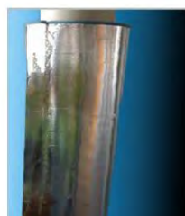
Tape along the longitudinal overlapped length
