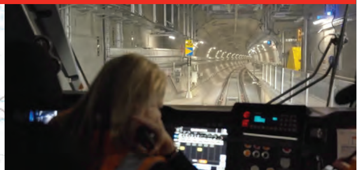
Test trains in the Metro Tunnel after three weeks of initial trials now reach full speed (80 km/h) to ensure everything is safe and ready for passengers. (Image credit: Rail Projects Victoria)
