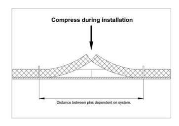
To achieve this, the anchor pattern is designed to introduce an overlap. The blanket strips are impaled symmetrically over the pins and thus overlap the neighbouring strip. The two adjacent strips at the overlap are pulled outwards together, aligned centrally and then pushed back into position forming a neat and compressed butt joint.
